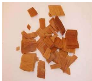
figure 4.1.17b - Chips after short pre-treatment at 150°. Wood yield 99%. Dry matter content 43%.
