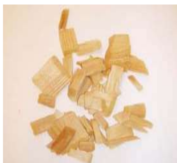
Figure 4.1.17a – Fresh chips. Dry matter content 57%.
