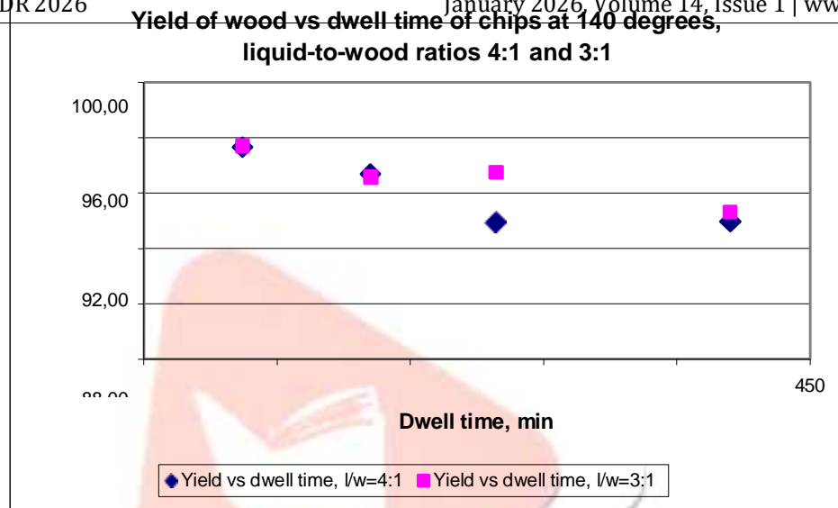
Figure 4.1.4 – The yield of wood after hot water pre-treatment of wood chips at 140 degree C and liquid-to-wood ratio 4:1 and 3:1 for different dwell times of the chips.
