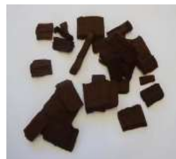
figure 4.1.17c - Chips after deep pre-treatment at 150degree C. Wood yield 88%. Dry matter content 37%.
