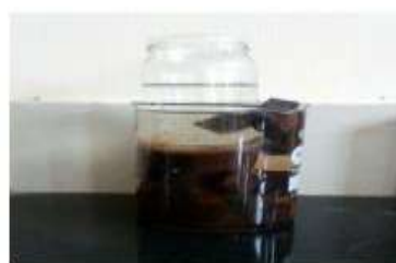
Wooden samples soaked in water for maximum absorption
