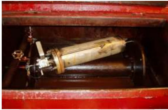
Figure 3 - Autoclave in the glycol bath
